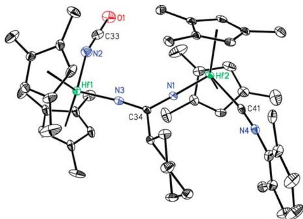
**Figure 5.** Molecular structure of **10** at 30% probability ellipsoids. Hydrogen atoms and one molecule of benzene solvate omitted for clarity. Selected bond distances (Å): Hf(2)–N(1) = 1.932(4), Hf(1)–N(3) = 1.936(5), N(1)–C(34) = 1.324(7), and N(3)–C(34) = 1.311(7).
