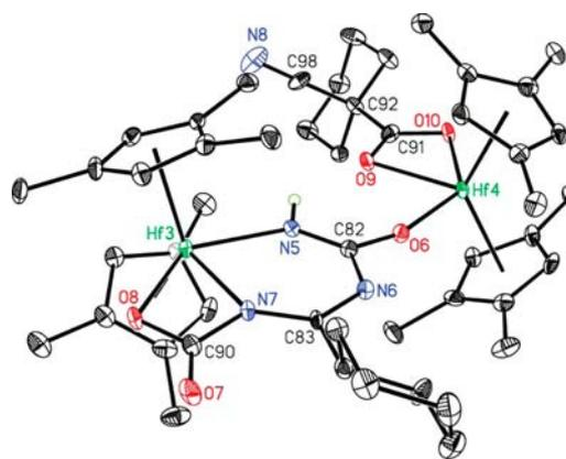
**Figure 8.** Molecular structure of one of two independent molecules of **15** at 30% probability ellipsoids. Hydrogen atoms (except that attached to N5) and one molecule of toluene solvate omitted for clarity. Selected bond distances (Å): N(5)–C(82) = 1.279(8), N(6)–C(82) = 1.395(7), N(6)–C(83) = 1.327(8), N(7)–C(83) = 1.351(7), N(7)–C(90) = 1.387(8), Hf(3)–N(5) = 2.235(5), and Hf(3)–N(7) = 2.199(5).
