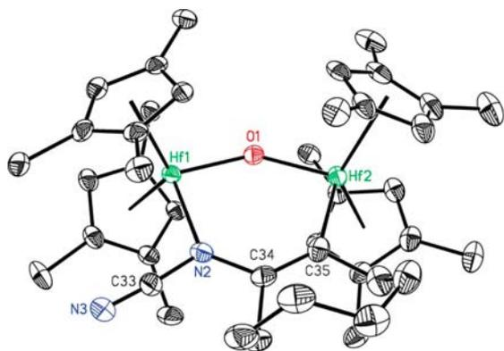
**Figure 3.** Molecular structure of **4** at 30% probability ellipsoids. Hydrogen atoms and one molecule of toluene omitted for clarity. Selected bond distances (Å): N(2)–C(33) = 1.152(8), N(3)–C(33) = 1.313(8), N(2)–C(34) = 1.489(8), and C(34)–C(35) = 1.322(9).
